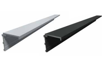
DS-PF Perimeter/Fascia Profile Fixes to side of joist to allow vertical fixing of boards where step/fascia detail is required. Finish: Mill finish or powder coated
